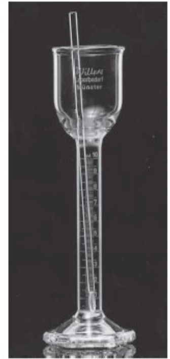
Fig. 9.1 Wide-mouthed, specially-made glass measuring cylinder and glass rod for the collection and mixing of semen and measurement of its volume
